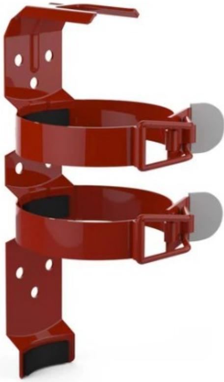
The 818S is an aviation bracket for 2 1/2lb and 3lb fire extinguishers, made of steel with a red, powder-coated finish. Key specifications include: Its compatibility with specific models like B385, C352, C354, B417, B403, and B410. Its support for a 2 1/2lb. tank weight and 3-inch tank diameter, meeting ASTM B117 and UL listed standards.
