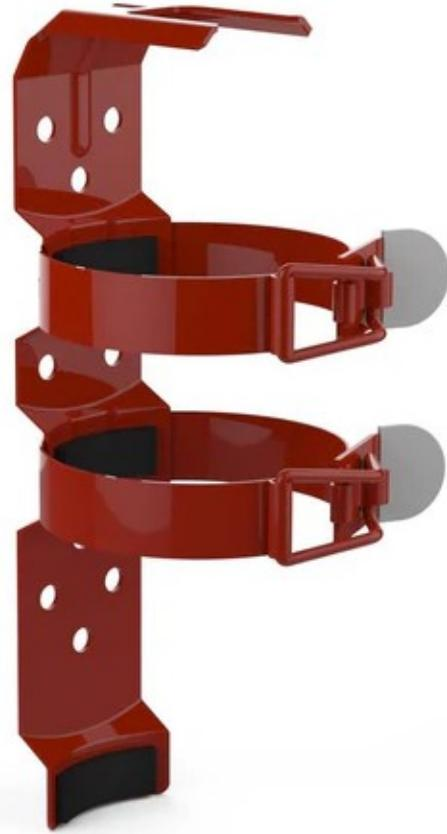
The 818S is an aviation bracket for 5lb fire extinguishers, made of steel with a red, powder-coated finish. Key specifications include: Its compatibility with specific models like B386, B355, B394, B402, B500, B409, B453 and B479. Its support for a 5lb. and 5.5lb tank weight and 4.25-inch tank diameter, and meeting ASTM B117 and UL listed standards.
