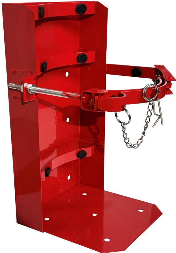
The 811G is a heavy duty bracket for 20lb and 30lb fire extinguishers, made of galvanized steel with a red, powder-coated finish. Key specifications include: Its compatibility with specific models like 567, 568, 569, 589, 591, 332, B570, B571, 715, 718, 792 and 796. Its support for a 30lb. tank weight and a 7 3/4 to 8-inch tank diameter, meeting ASTM B117 and UL listed standards.
