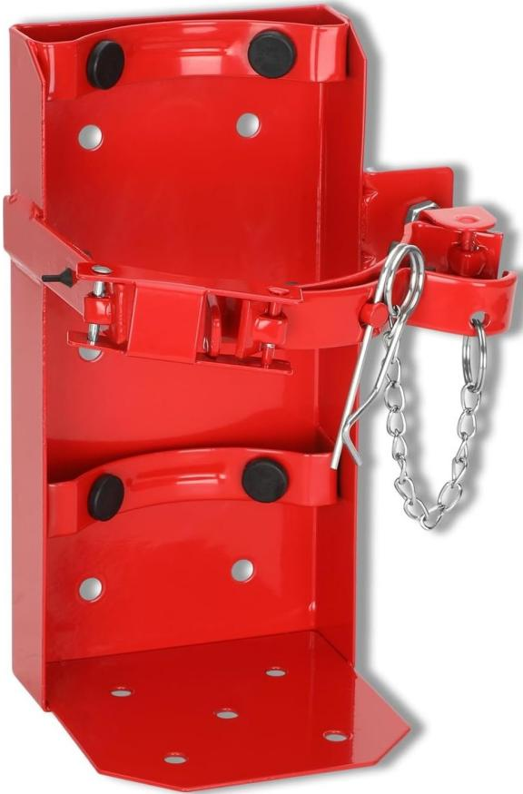
The 809G is a marine/vehicle bracket for 10lb fire extinguishers, made of galvanized steel with a red, powder-coated finish. Key specifications include: its compatibility with specific models like B369, B371, B443, B461, B456, B441, B462, B447, B457, B460, 322, 720, 721 and 722 its support for a 10lb. tank weight and a 5 to 5.25-inch tank diameter, meeting ASTM B117 and UL listed standards.
