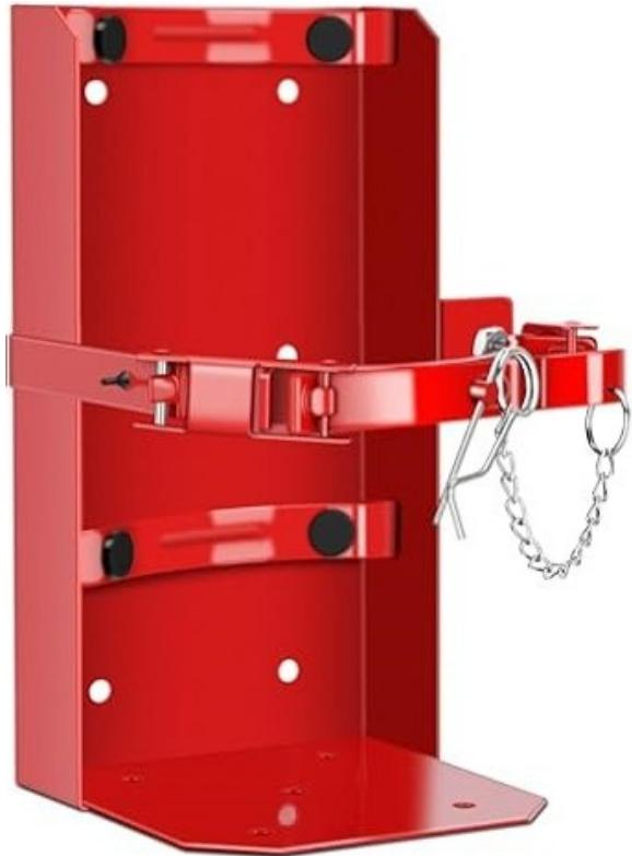
The 810G is a heavy duty bracket for 13.2lb to 20lb fire extinguishers, made of galvanized steel with a red, powder-coated finish. Key specifications include: Its compatibility with specific models like 240, 254, 250, B260, 361, A411, 423, A412, 408, A413, 415, 330, 331, 592, 594, 595, 599, 581, 585, 580, 584, 564, 566, 760, 761 and 762. Its support for a 13.2lb. and 20lb tank weight and 7-inch tank diameter, and meeting ASTM B117 and UL listed standards.
