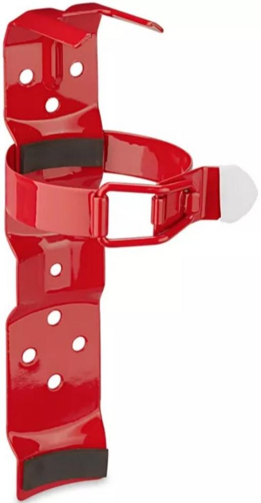
The 817A is a vehicle bracket for 2.5 lb. dry chemical fire extinguishers, made of steel with a red, powder-coated finish. Key specifications include: its compatibility with specific models like B403, B417, and C352TS, its support for a 2.5 lb. tank weight and 3-inch tank diameter, and meeting ASTM B117 and UL listed standards.
